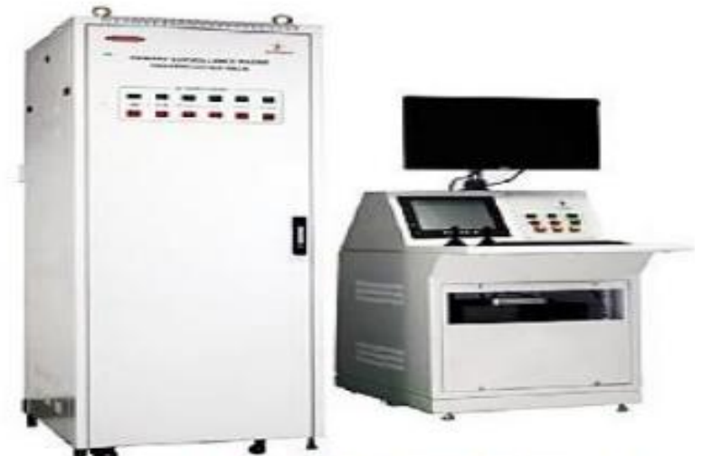
Designed and developed Primary Surveillance Radar for coastal surveillance for the Indian government space organization
